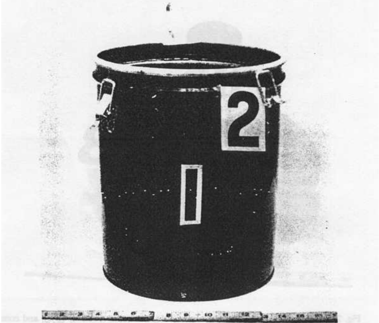
Fig. 2-21. Filter container (#1) showing latches (#2) for lid and hose (#3) around top.
