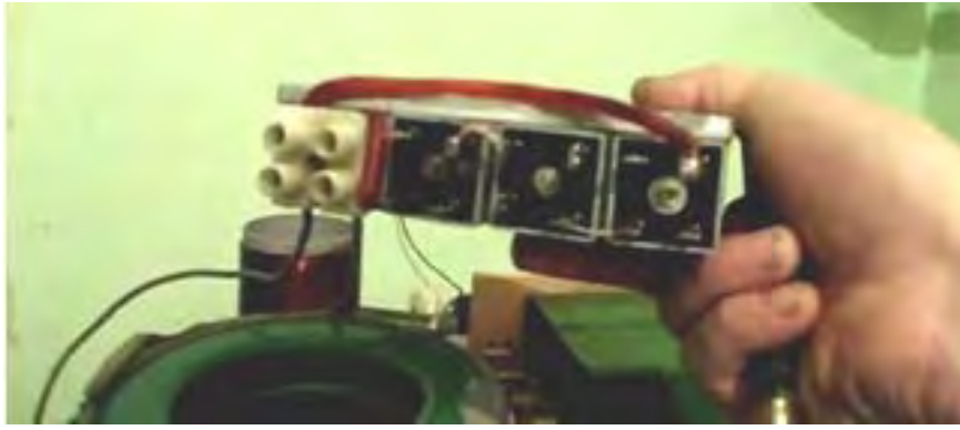
Three 1000V diode bridges can be connected to withstand a voltage of 6 kV.
