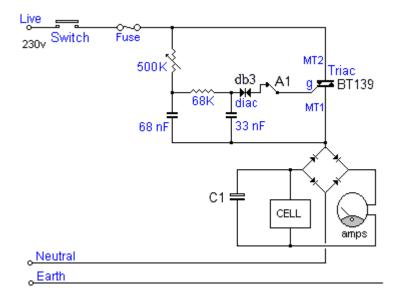
The first part of David Quirey's circuit acts very much like a dimmer light switch. The 230-volt AC mains is fed through an On/Off switch and then an ordinary mains fuse. The current flow on through the circuit is blocked by the BT139 triac until it receives a pulse from the db3 diac (which is a component specifically designed to feed pulses to a triac).
