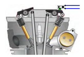
An alternative is to attach a strong permanent magnet to the rocker arm, using epoxy resin, and then position a solid state "Hall-effect" sensor so that it triggers the delay before the spark is generated.
