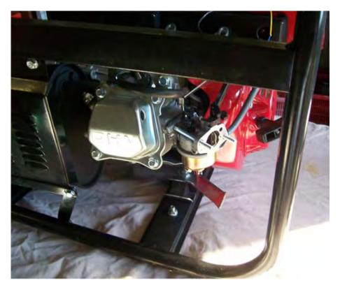
This allows access to the carburettor which is then removed as it will not be used:
