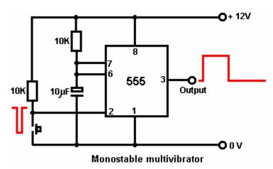
If you are not at all familiar with electronic circuits, then take a look at the beginner's electronics tutorial found in the Appendix as that explains how circuitry works and how to build any simple circuit from scratch. We can use two of these circuits, the first to give the adjustable delay and the second to give a brief pulse to the ignition circuit to generate the spark:
