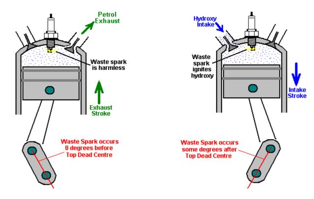
we definitely do not want that to happen, so it is very important that we suppress that additional "waste" spark. So, this leaves us with two engine adjustments: timing delay and waste spark elimination. There are various ways in which these can be done and as each engine design is different, it is difficult to cover every possibility. However, there is a technique which can be used with many engines and which deals with both issues at the same time.
