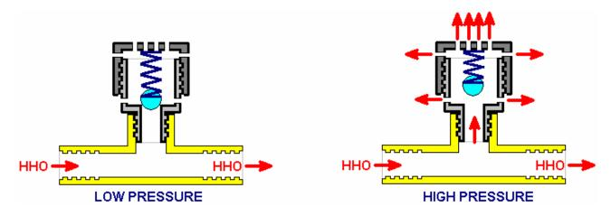
When the gas pressure drops again, the spring pushes the roller ball down to seal off the pressurerelease holes.
