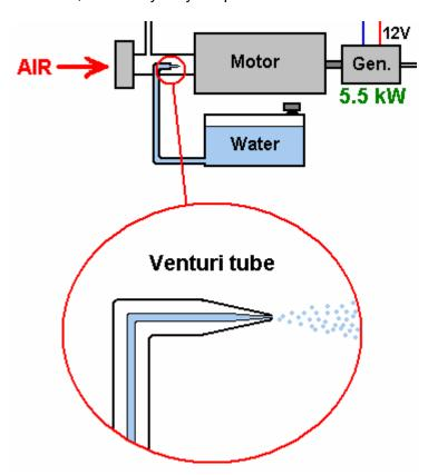
It is just a pipe which tapers to a point and which has a very small nozzle. As the engine draws in the air/HHO mix on it's intake stroke, the mixture rushes past the nozzle of the Venturi tube. This creates an area of lower pressure outside the nozzle and causes water to exit through the nozzle in a spray of very fine droplets. Some perfume spray bottles use this method as it is both cheap and effective.
