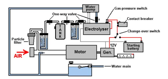
This arrangement is perfectly capable of running a standard generator without the use of any fossil fuel. It should be noted that while no fossil fuel needs to be bought to run this generator system, the electrical output is far from free and is actually quite expensive as there is the purchase cost of the generator, the electrolyser and the minor additional equipment. Also, generators have a definite working life and so will need to be refurbished or replaced.
