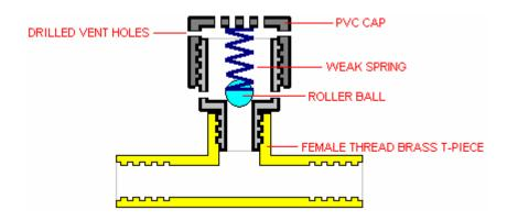
The ball is held in place by the spring allowing the HHO to flow past it, but if a sudden increase in pressure should occur, then the ball is forced upwards, opening a path to the many holes drilled in the plastic fittings:
