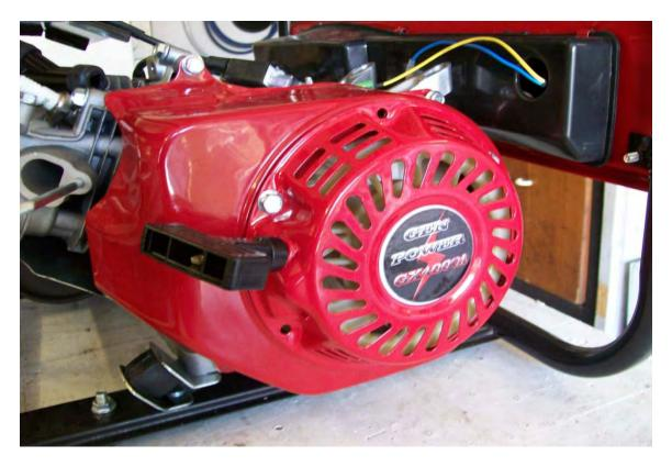
The manual Pull-start and the generator cover are now removed. It is only necessary to remove four of the bolts to take the cover off:
