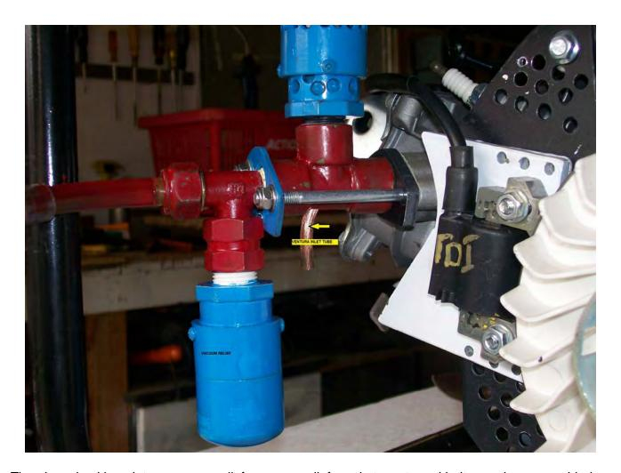
The pipes, backing plate, pressure-relief, vacuum-relief, gaskets, nuts and bolts are then assembled as shown above. Most of the pressure-relief valve components shown in the photograph have been painted, which happens to conceal the different materials being used.
