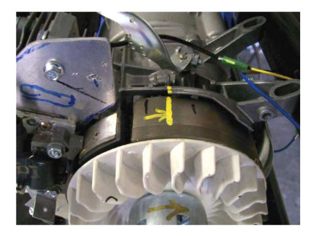
5. Next comes a bit of arithmetic. The diameter of the flywheel is 180 mm which means that it's circumference is  $3.14159 \times 180 = 565.5 \text{ mm}$  and as there are 360 degrees in each rotation of the flywheel, then the outside edge of the flywheel will move 1.57 mm for each of those degrees.
