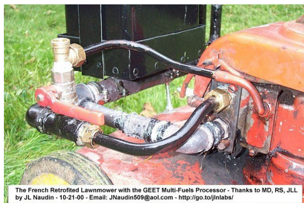
A close view of the Intake/Exhaust connection of the engine
