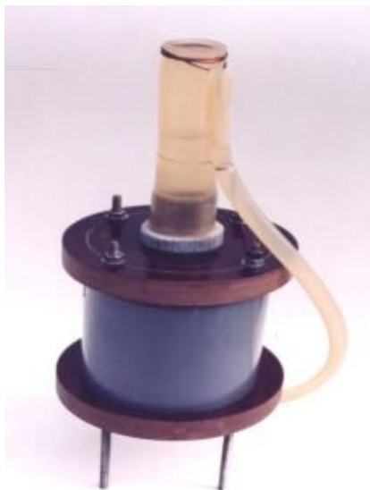
Fig. 1. Model of a low current cell of the electrolyzer (at the stage of patenting)
